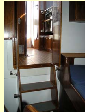
Ladder and engine access, front cabin. After removal of the ladder, one can open a second door. A trap door of floor in the saloon also gives access to the engine room. One will note "bedside tables" to the head of the bunks.
